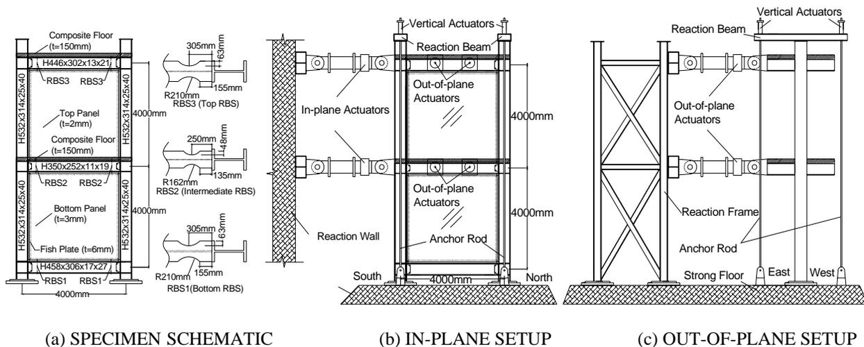
FIGURE 1 – SPECIMEN AND TEST SETUP
